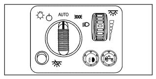
The exterior lamp control is located on the instrument panel on the left side of the steering wheel. (Exterior Lamps): Turn the knob, located to the right of this symbol, to choose one of the four exterior lamp positions.
